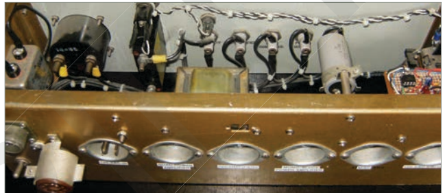
Photo 7: An inside view of the rear of the power distribution showing front-panel fuses
