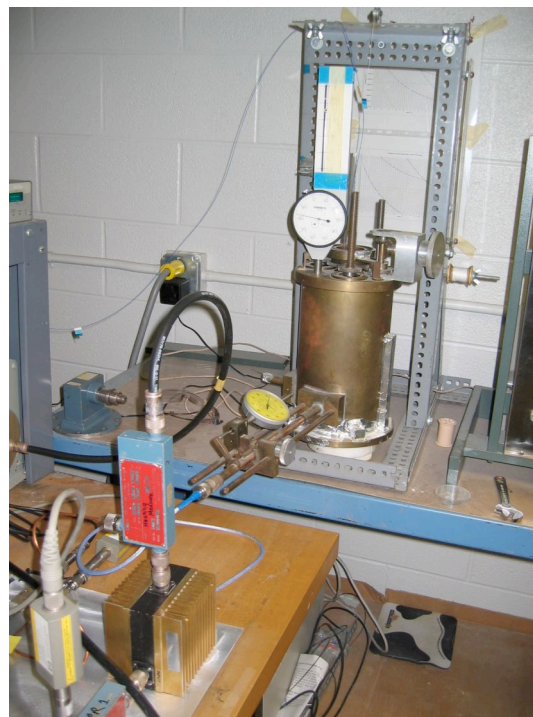
Figure 3. Illustration of the single-mode cavity. The switch system is in the lower-left corner of the figure.
